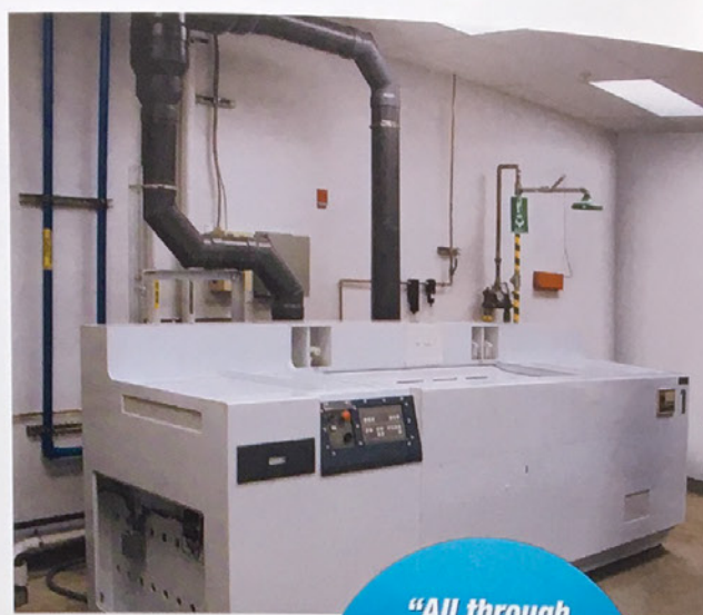
Used process water from Ebara's wet benches is reclaimed, conserving water resources.
